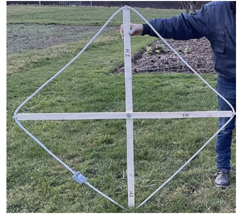
Figure 6 – 1m Square Version of the Loop Showing the location of the connection box
